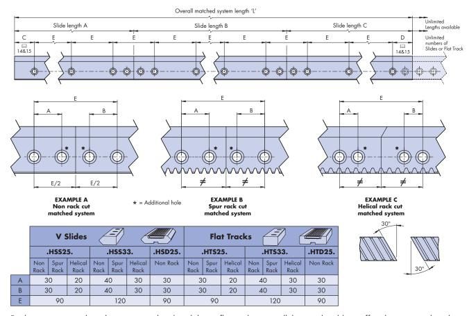
For best running quality when using single edge slides or flat tracks in parallel, it is advisable to offset the joints so they do not coincide. It is also important to ensure that slides and tracks overlap any joints in the back plates or beams where these have been supplied in joined condition for long length requirements. Such applications should be discussed with Hepco.
